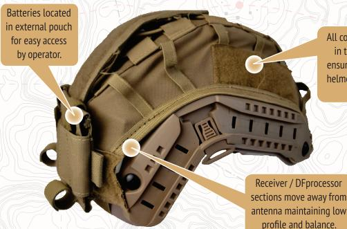
All components housed in the helmet cover ensuring no changes to helmet's ballistic/bump protection.
